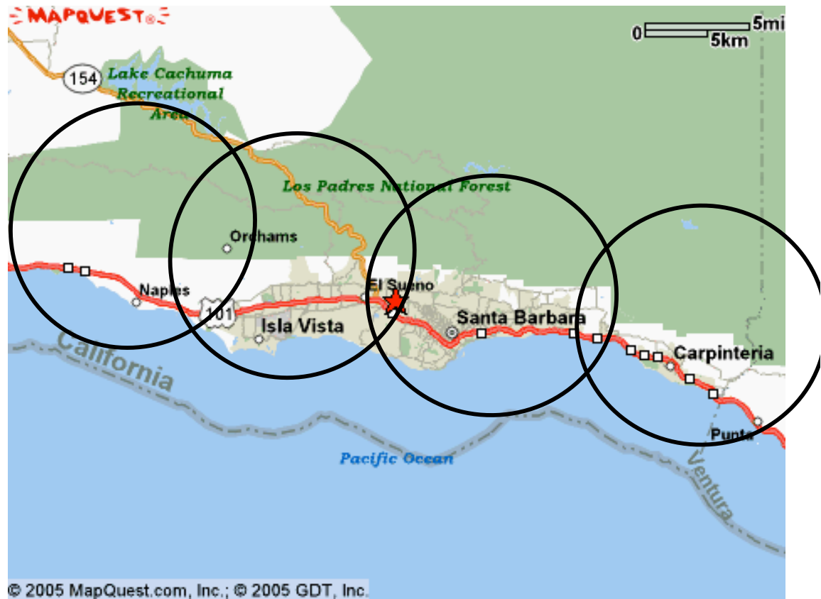
Figure 1: A new wireless system covers a large area with a few cell sites.
