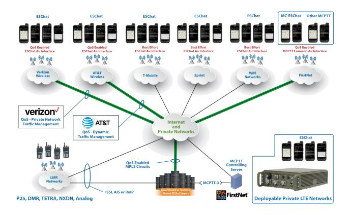
It is sometimes the case that the mission calls for a field-deployable or standalone push-to-talk system and wireless data network. These instances are common in the mining and utility industries where the remote locations are not serviced by traditional wireless carriers. In public safety, deployable networks can be ideally suited for use in Search and Rescue (SAR) and remote fire-fighting activities.
