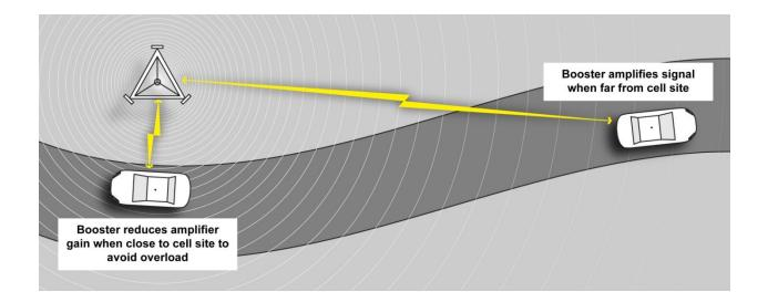
As you approach the cell site, less and less boost of your phone's signal is required. In this situation, the amplifier reduces the gain, or if necessary, shuts off completely. Thus at no time is the cell site overloaded with too strong a signal. Then, as you move away from the site and signal amplification is required, the booster comes back on (if it shut down) and continually varies its gain for optimal performance.
