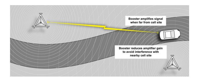
By continuously monitoring the signal strength of nearby cell sites, the Wilson cell phone booster adjusts the transmitting signal gain (amplification) to avoid the possibility of interference with the nearby cell site, even though that site may use different frequencies or technologies. As you move away from the nearby cell site, the booster can increase signal amplification to give you the best possible connection to your distant cell site without ever interfering with the nearby cell site.
