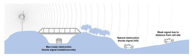
Poor signal strength has another effect on your phone's performance. Wireless networks are designed to minimize the amount of power necessary for your phone to communicate with the cell site. The closer you are to a site, the less power required from your phone and the longer your battery life. Conversely, the further you are from a cell site, or the more obstacles between your phone and the cell site, the more power the phone must use to communicate, and this will shorten its battery life
