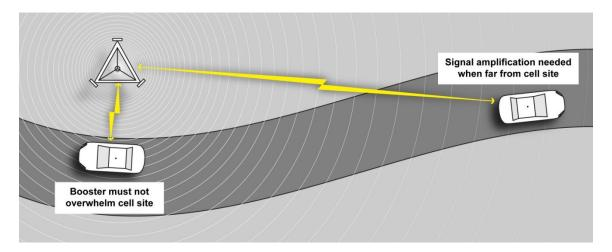
• Avoiding interference to adjacent cell sites. A more subtle variation of the above occurs when your cell phone is communicating with a distant cell site, but there is another cell site (operated by a different service provider) close by. There is a possibility that the booster could cause interference to the other network operators' cell site. If the booster transmits a strong signal in order to reach the distant site, it could potentially interfere with the nearby cell site.
