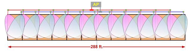
The output of the couplers on the waveguide connect through short cables to inexpensive, specially designed 90-degree beamwidth spatial stream directional, room antennas – one antenna per spatial stream per room or area in a system. Two or more SS antennas illuminate each room to provide ideal, local, MIMO signals. Note the physical separation of spatial signal antennas in each room to create a fixed, stable, time differential.
